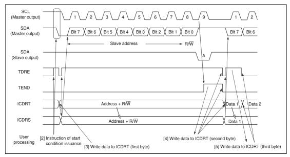
Figure 17.5 Master Transmit Mode Operation Timing (1)
