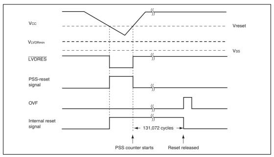
Figure 19.4 Operating Timing of LVDR Circuit
