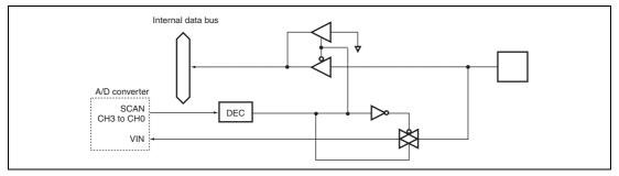
Figure B.24 Port B Block Diagram (PB5 to PB0)
