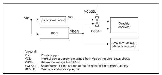
Figure 19.1 Block Diagram around BGR
