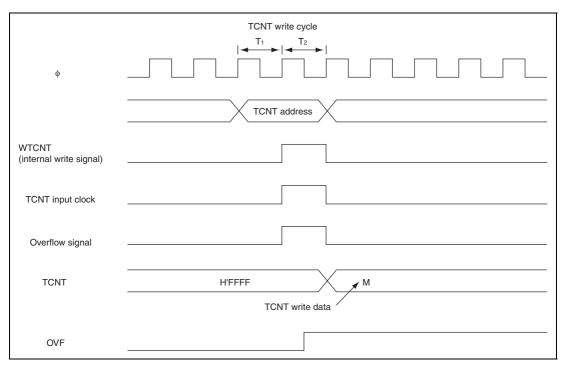
Figure 13.55 Contention between TCNT Write and Overflow
