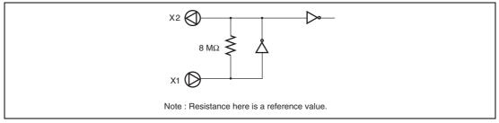
Figure 5.15 Block Diagram of Subclock Oscillator
