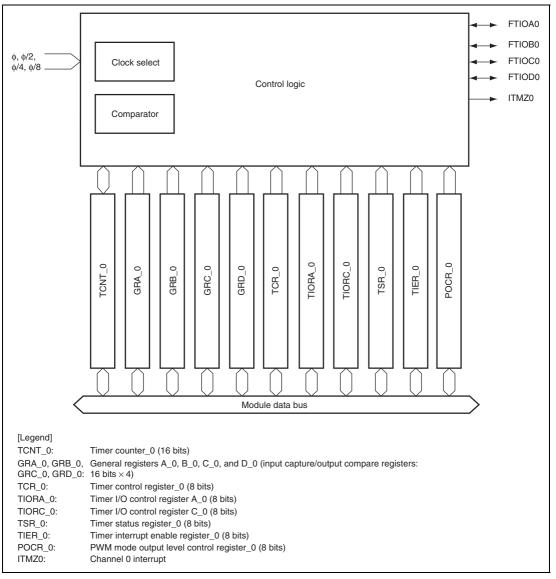
Figure 13.2 Timer Z (Channel 0) Block Diagram
