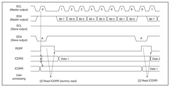
Figure 17.11 Slave Receive Mode Operation Timing (1)
