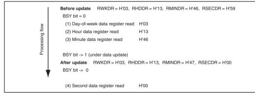
Figure 10.4 Example: Reading of Inaccurate Time Data
