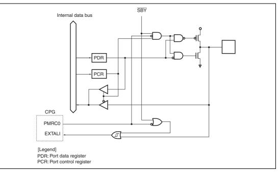
Figure B.26 Port B Block Diagram (PC0)
