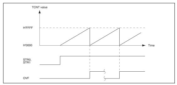
Figure 13.8 Free-Running Counter Operation
