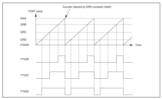
Figure 13.23 Example of PWM Mode Operation (2)
