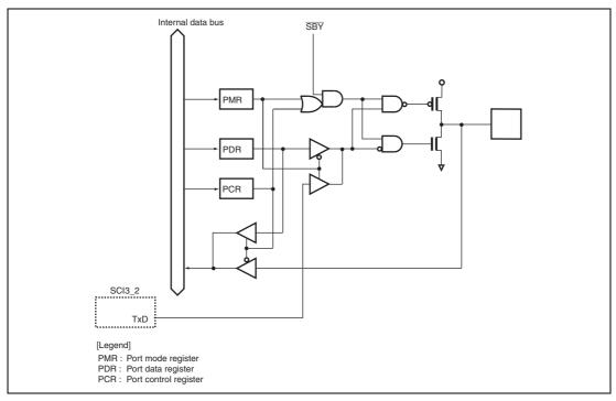
Figure B.19 Port 7 Block Diagram (P72)
