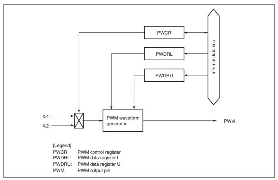
Figure 15.1 Block Diagram of 14-Bit PWM
