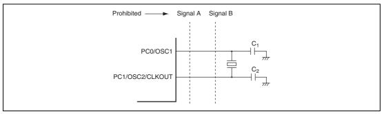
Figure 5.19 Example of Incorrect Board Design
