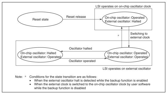
Figure 5.2 State Transition of System Clock
