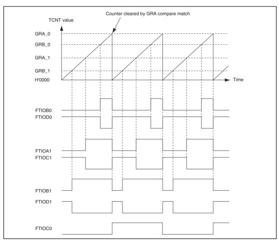
Figures 13.27 and 13.28 show examples of operation in reset synchronous PWM mode.
