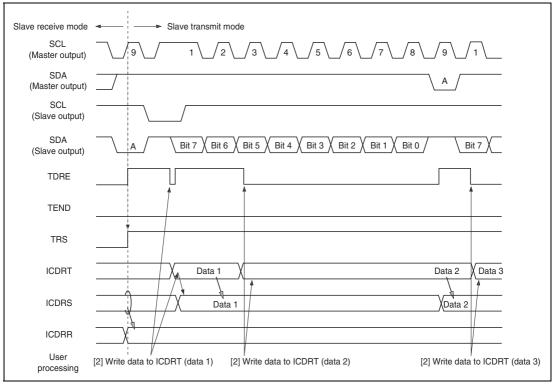
Figure 17.9 Slave Transmit Mode Operation Timing (1)
