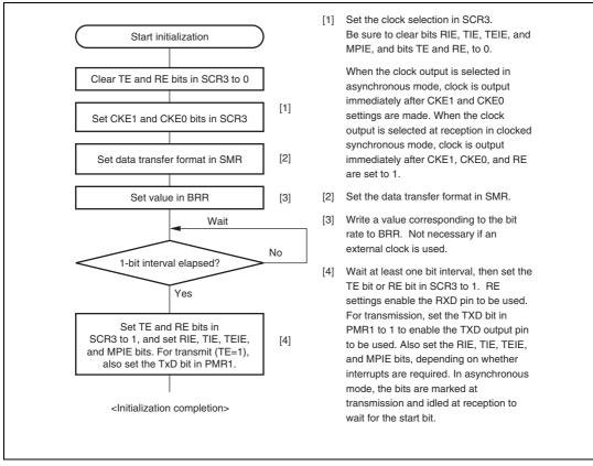
Figure 16.4 Sample SCI3 Initialization Flowchart
