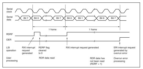
Figure 16.12 Example of SCI3 Reception in Clock Synchronous Mode
