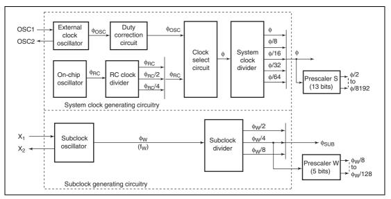
Figure 5.1 Block Diagram of Clock Pulse Generator
