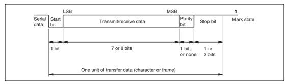
Figure 16.2 Data Format in Asynchronous Communication
