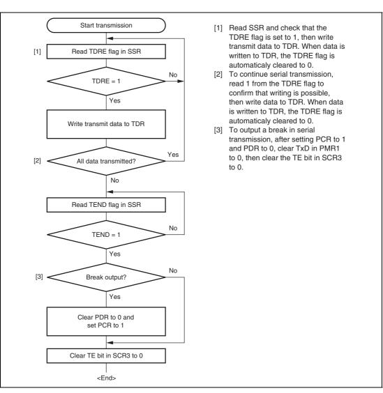
Figure 16.6 Sample Serial Transmission Data Flowchart (Asynchronous Mode)
