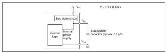
Figure 20.1 Power Supply Connection when Internal Step-Down Circuit is Used
