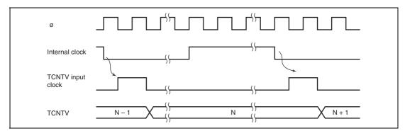
Figure 12.2 Increment Timing with Internal Clock
