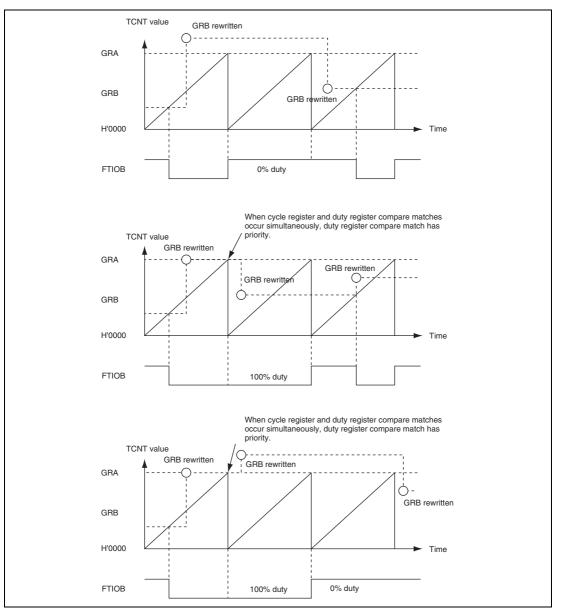
Figure 13.24 Example of PWM Mode Operation (3)
