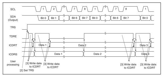
Figure 17.14 Transmit Mode Operation Timing
