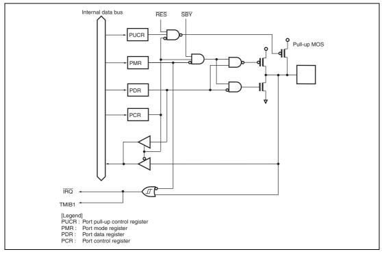
Figure B.3 Port 1 Block Diagram (P15)
