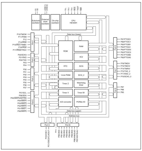
Figure 1.1 Block Diagram of H8/36077 Group
