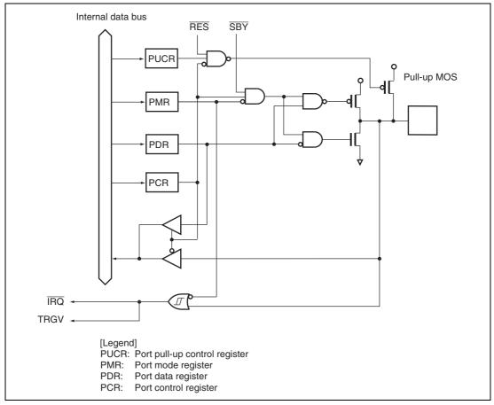
Figure B.1 Port 1 Block Diagram (P17)
