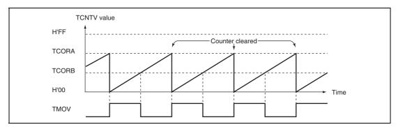
Figure 12.9 Pulse Output Example
