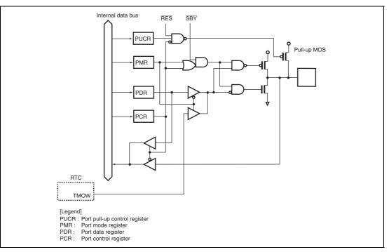
Figure B.6 Port 1 Block Diagram (P10)
