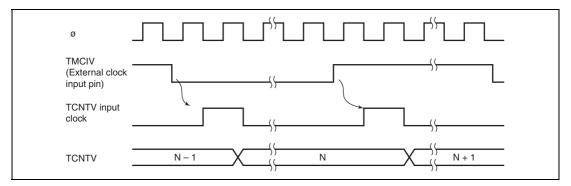
Figure 12.3 Increment Timing with External Clock
