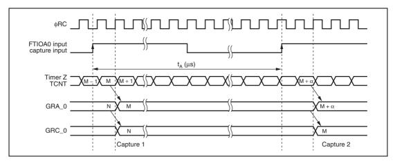
Figure 5.10 Timing Chart of Trimming of On-Chip Oscillator Frequency
