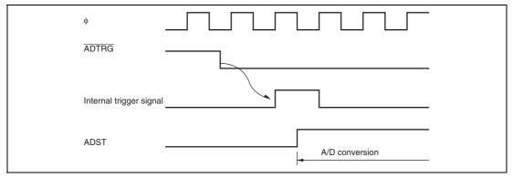
Figure 18.3 External Trigger Input Timing
