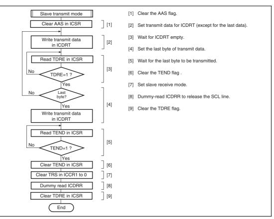
Figure 17.19 Sample Flowchart for Slave Transmit Mode
