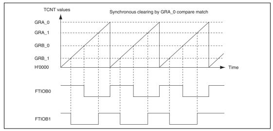
Figure 13.20 Example of Synchronous Operation
