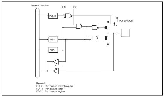
Figure B.4 Port 1 Block Diagram (P12)
