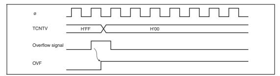
Figure 12.4 OVF Set Timing
