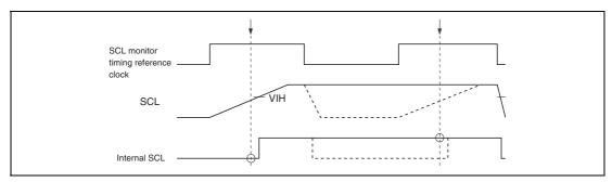
Figure 17.21 The Timing of the Bit Synchronous Circuit
