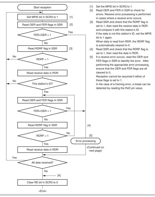
Figure 16.17 Sample Multiprocessor Serial Reception Flowchart (1)
