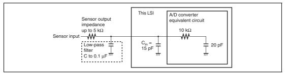
Figure 18.6 Analog Input Circuit Example
