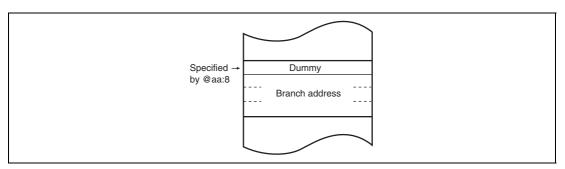
Figure 2.8 Branch Address Specification in Memory Indirect Mode
