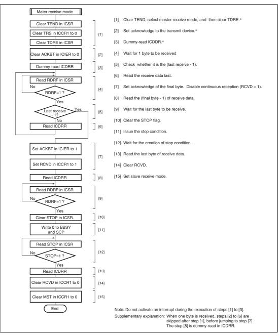
Figure 17.18 Sample Flowchart for Master Receive Mode
