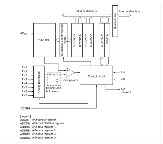
Figure 18.1 Block Diagram of A/D Converter
