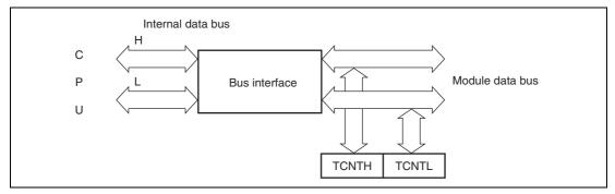
Figure 13.5 Accessing Operation of 16-Bit Register (between CPU and TCNT (16 bits))
