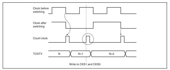
Figure 12.13 Internal Clock Switching and TCNTV Operation
