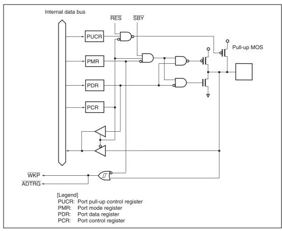
Figure B.13 Port 5 Block Diagram (P55)
