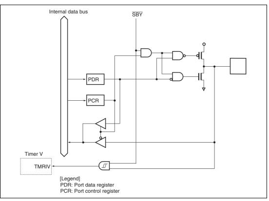
Figure B.18 Port 7 Block Diagram (P74)
