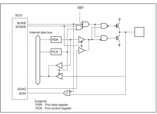
Figure B.10 Port 2 Block Diagram (P20)
