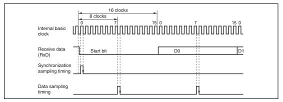
Figure 16.19 Receive Data Sampling Timing in Asynchronous Mode
