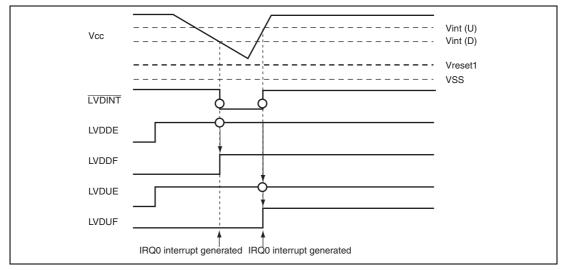
Figure 19.5 Operational Timing of LVDI Circuit
