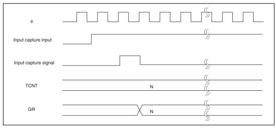
Figure 13.18 Input Capture Signal Timing
