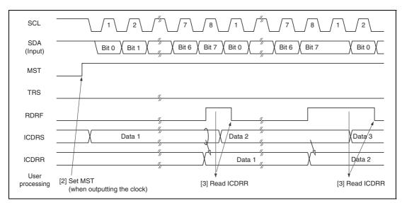
Figure 17.15 Receive Mode Operation Timing
