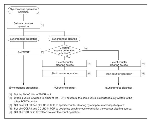
Figure 13.19 Example of Synchronous Operation Setting Procedure
