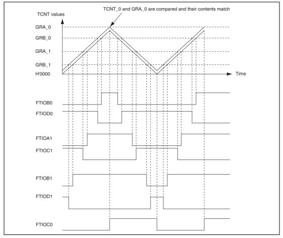
Figure 13.31 Example of Complementary PWM Mode Operation (1)
