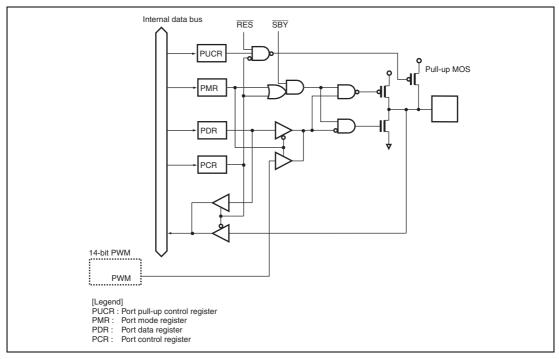
Figure B.5 Port 2 Block Diagram (P11)
