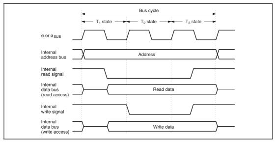
Figure 2.10 On-Chip Peripheral Module Access Cycle (3-State Access)
