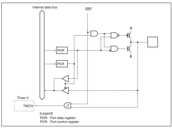
Figure B.17 Port 7 Block Diagram (P75)
