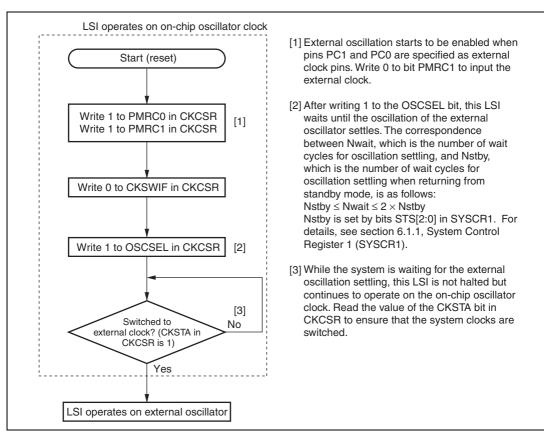
Figure 5.4 Flowchart of Clock Switching with Backup Function Disabled (1) (From On-Chip Oscillator Clock to External Clock)
