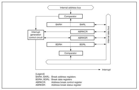
Figure 4.1 Block Diagram of Address Break
