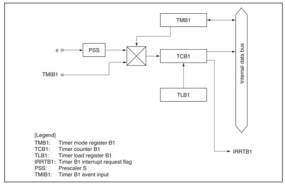
Figure 11.1 Block Diagram of Timer B1
