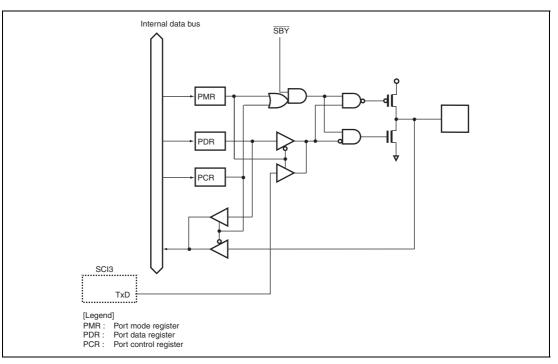
Figure B.8 Port 2 Block Diagram (P22)
