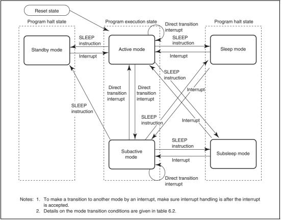
Figure 6.1 Mode Transition Diagram
