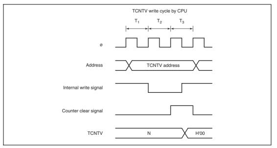
Figure 12.11 Contention between TCNTV Write and Clear
