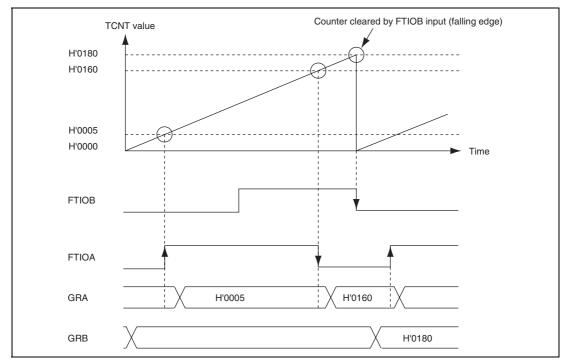
Figure 13.17 Example of Input Capture Operation
