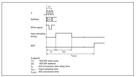
Figure 18.2 A/D Conversion Timing
