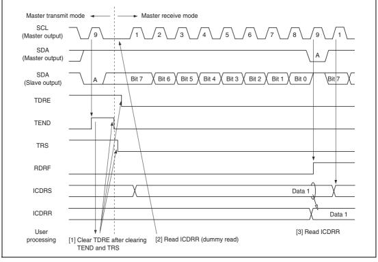
Figure 17.7 Master Receive Mode Operation Timing (1)
