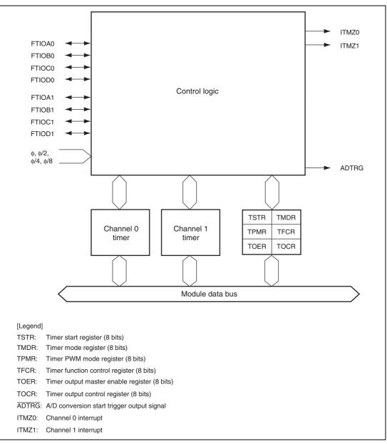
Figure 13.1 Timer Z Block Diagram
