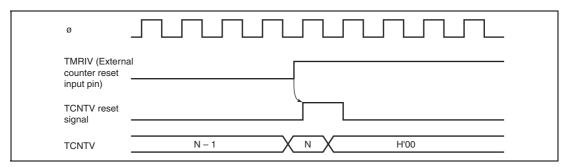
Figure 12.8 Clear Timing by TMRIV Input
