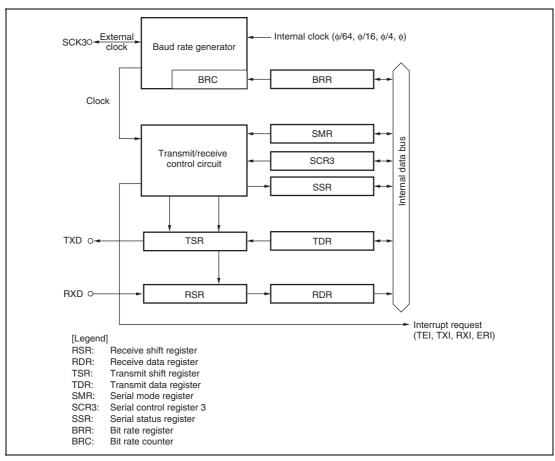
Figure 16.1 Block Diagram of SCI3
