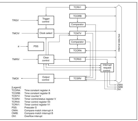
Figure 12.1 Block Diagram of Timer V
