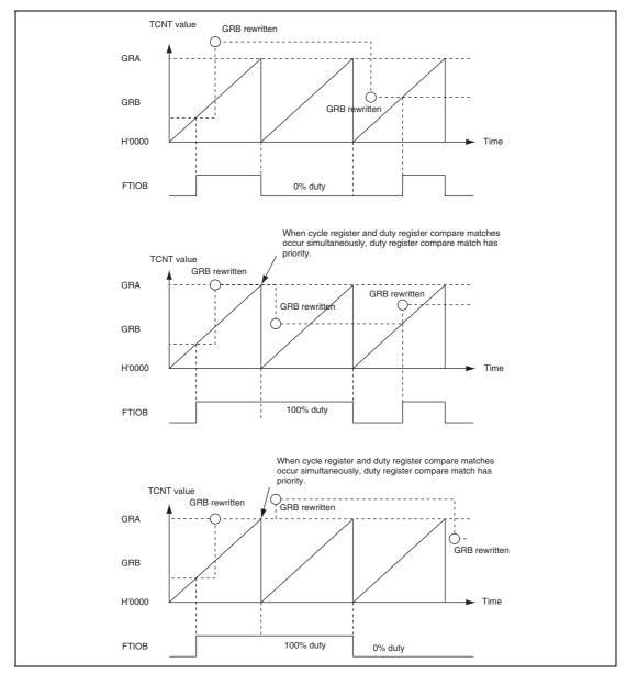
Figure 13.25 Example of PWM Mode Operation (4)
