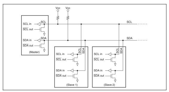
Figure 17.2 External Circuit Connections of I/O Pins
