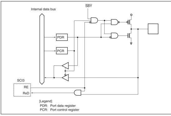
Figure B.9 Port 2 Block Diagram (P21)
