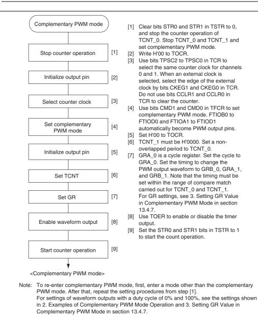
Figure 13.29 Example of Complementary PWM Mode Setting Procedure
