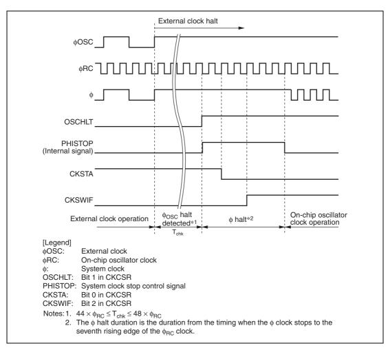
Figure 5.8 External Oscillation Backup Timing
