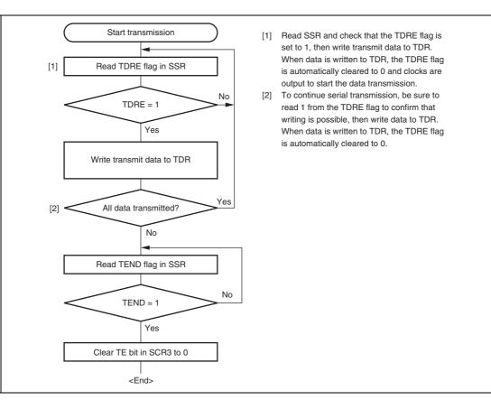
Figure 16.11 Sample Serial Transmission Flowchart (Clock Synchronous Mode)
