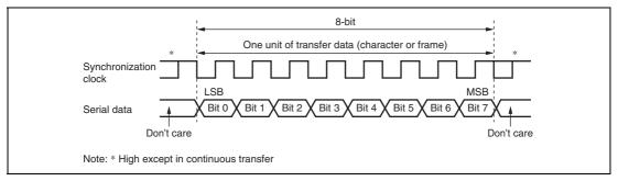
Figure 16.9 Data Format in Clock Synchronous Communication
