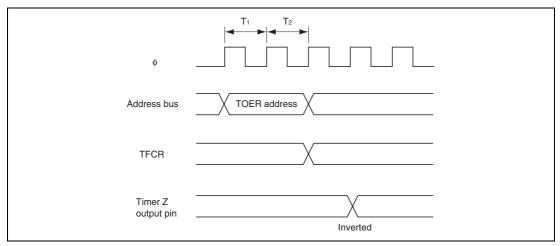
Figure 13.46 Example of Output Inverse Timing of Timer Z by Writing to TFCR
