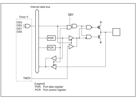
Figure B.16 Port 7 Block Diagram (P76)
