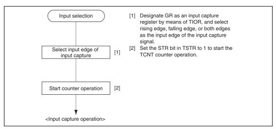
Figure 13.16 Example of Input Capture Operation Setting Procedure
