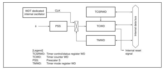
Figure 14.1 Block Diagram of Watchdog Timer
