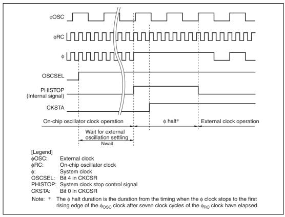
Figure 5.6 Timing Chart of Switching from On-Chip Oscillator Clock to External Clock
