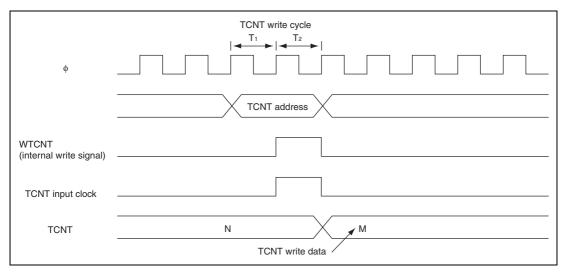
Figure 13.53 Contention between TCNT Write and Increment Operations
