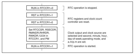
Figure 10.3 Initial Setting Procedure
