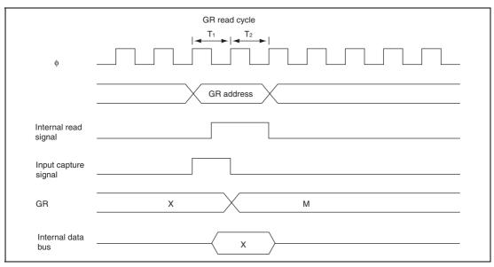
Figure 13.56 Contention between GR Read and Input Capture
