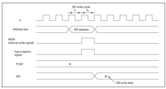
Figure 13.58 Contention between GR Write and Input Capture
