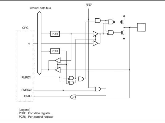
Figure B.25 Port B Block Diagram (PC1)
