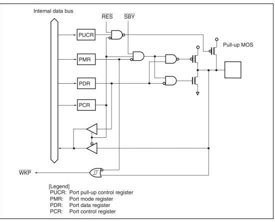
Figure B.14 Port 5 Block Diagram (P54 to P50)
