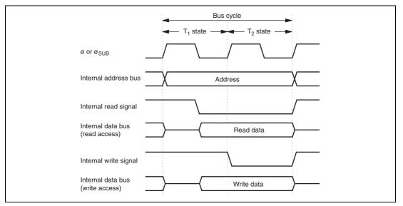
Figure 2.9 On-Chip Memory Access Cycle
