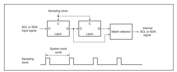
Figure 17.16 Block Diagram of Noise Filter
