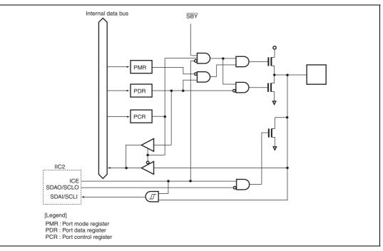
Figure B.12 Port 5 Block Diagram (P57, P56)
