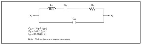
Figure 5.17 Equivalent Circuit of 32.768-kHz Crystal Resonator
