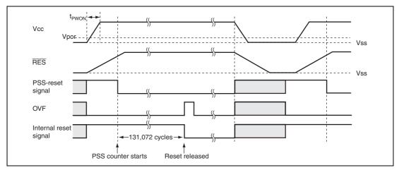
Figure 19.3 Operational Timing of Power-On Reset Circuit
