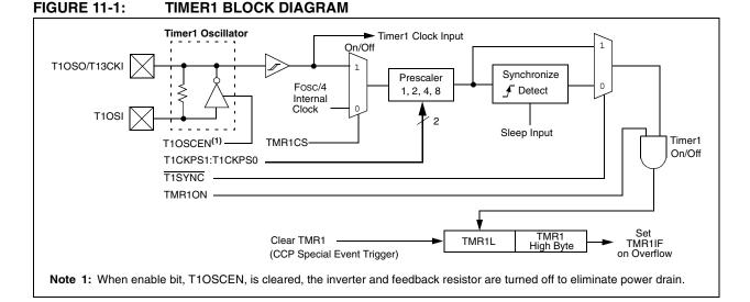
cycle (Fosc/4). When the bit is set, Timer1 increments on every rising edge of the Timer1 external clock input
