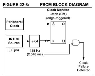
Clock failure is tested for on the falling edge of the sample clock. If a sample clock falling edge occurs while CM is still set, a clock failure has been detected (Figure 22-4). This causes the following:
