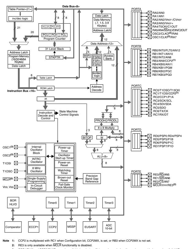
3: OSC1/CLKI and OSC2/CLKO are only available in select oscillator modes and when these pins are not being used as digital I/O. Refer to Section 2.0 "Oscillator Configurations" for additional information.
