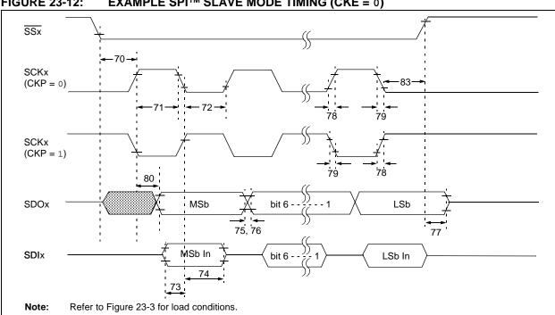
FIGURE 23-12: **EXAMPLE SPI™ SLAVE MODE TIMING (CKE = 0)**
