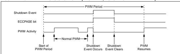
FIGURE 14-10: PWM AUTO-SHUTDOWN (PRSEN = 1, AUTO-RESTART ENABLED)
