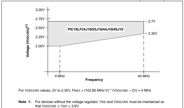
FIGURE 23-2: PIC18F45J10 FAMILY VOLTAGE-FREQUENCY GRAPH (INDUSTRIAL)
