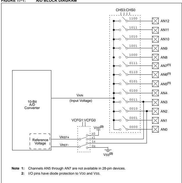
After the A/D module has been configured as desired, the selected channel must be acquired before the conversion is started. The analog input channels must have their corresponding TRIS bits selected as an input. To determine acquisition time, see Section 17.1 "A/D Acquisition Requirements". After this acquisi-
