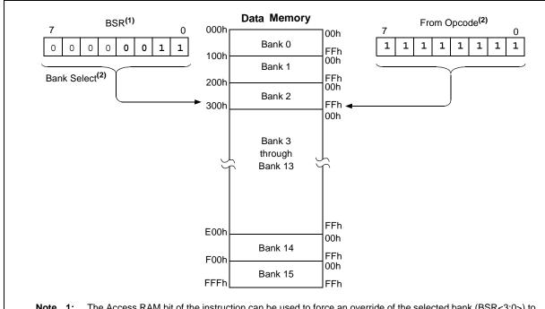
Note 1: The Access RAM bit of the instruction can be used to force an override of the selected bank (BSR<3:0>) to the registers of the Access Bank.
