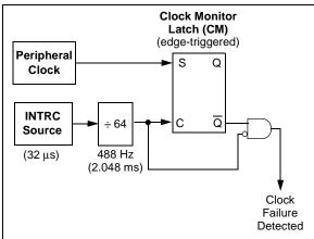
Clock failure is tested for on the falling edge of the sample clock. If a sample clock falling edge occurs while CM is still set, a clock failure has been detected (Figure 20-5). This causes the following:
