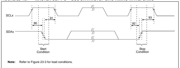
TABLE 23-20: MASTER SSP I<sup>2</sup>C™ BUS START/STOP BITS REQUIREMENTS
