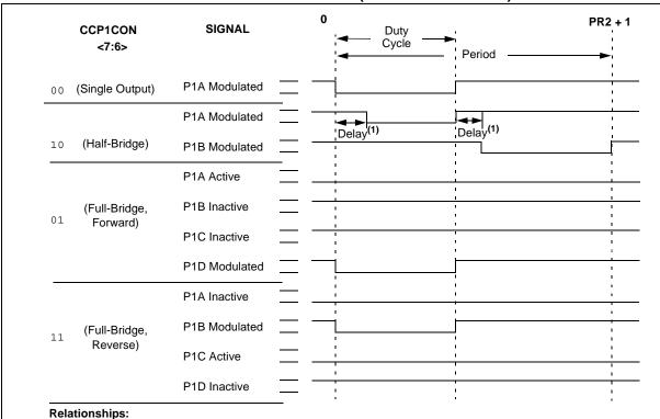
Note 1: Dead-band delay is programmed using the ECCP1DEL register (see Section 14.4.6 "Programmable
