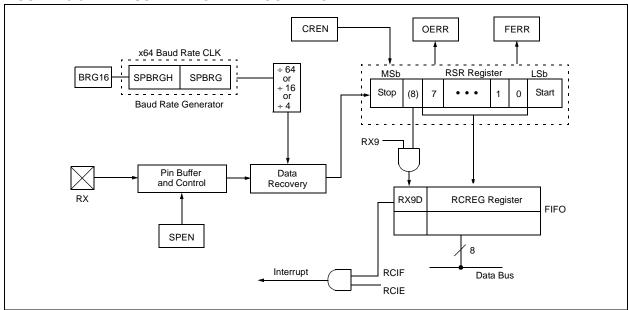
FIGURE 16-7: ASYNCHRONOUS RECEPTION
