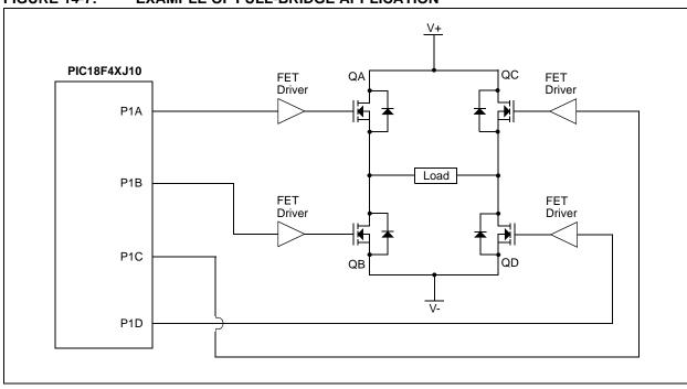
FIGURE 14-7: EXAMPLE OF FULL-BRIDGE APPLICATION
