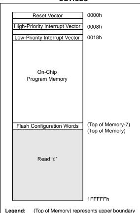
of on-chip program memory space (see Figure 5-1 for device-specific values). Shaded area represents unimplemented memory. Areas are not shown to scale.
