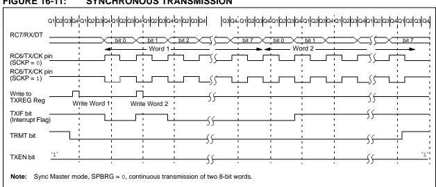
FIGURE 16-12: SYNCHRONOUS TRANSMISSION (THROUGH TXEN)
