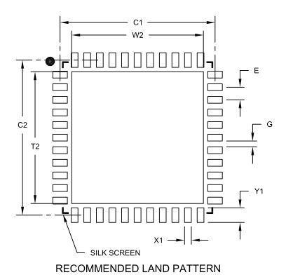
Units **MILLIMETERS Dimension Limits** MIN NOM MAX Contact Pitch 0.65 BSC Е Optional Center Pad Width W2 6.80 Optional Center Pad Length T2 6.80 C1 8.00 Contact Pad Spacing Contact Pad Spacing C2 8.00 Contact Pad Width (X44) X1 0.35 Contact Pad Length (X44) <u>Y1</u> 0.80 Distance Between Pads G 0.25
