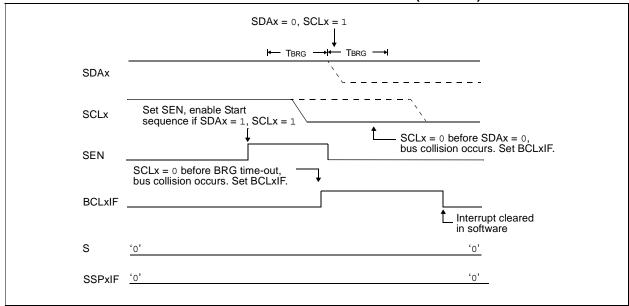
FIGURE 15-28: BRG RESET DUE TO SDAX ARBITRATION DURING START CONDITION
