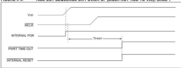
FIGURE 4-5: TIME-OUT SEQUENCE ON POWER-UP (MCLR NOT TIED TO VDD): CASE 2
