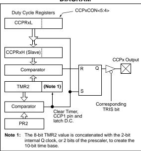
A PWM output (Figure 13-4) has a time base (period) and a time that the output stays high (duty cycle). The frequency of the PWM is the inverse of the period (1/period).
