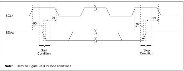
TABLE 23-18: I<sup>2</sup>C™ BUS START/STOP BITS REQUIREMENTS (SLAVE MODE)
