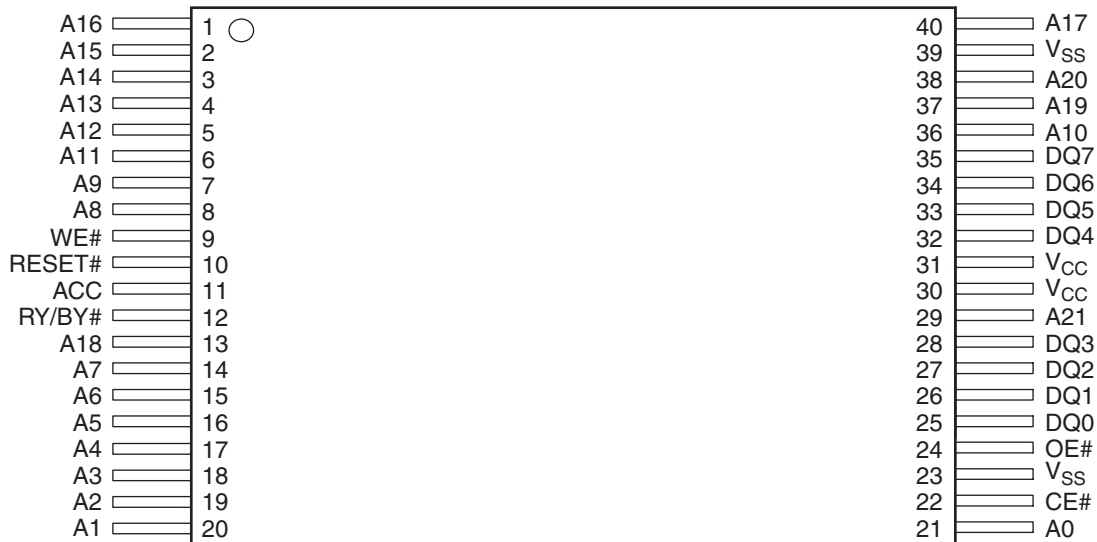
Figure 3.2 48-pin Standard TSOP
