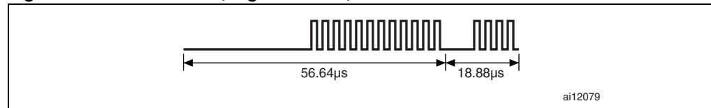
Figure 36. Start of frame, high data rate, one subcarrier x2
