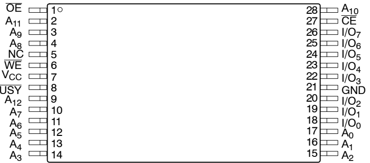
TSOP Package (8 mm x 13.4 mm) (H13)
