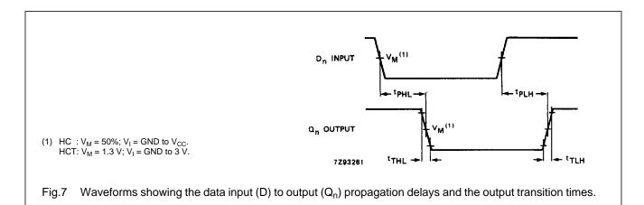
(1) HC:  $V_M = 50\%$ ;  $V_I = GND \text{ to } V_{CC}$ . HCT:  $V_M = 1.3 \text{ V}$ ;  $V_I = GND \text{ to } 3 \text{ V}$ .
