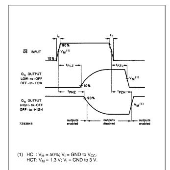
Fig.8 Waveforms showing the 3-state enable and disable times.
