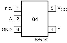
Fig.1 Pin configuration.
