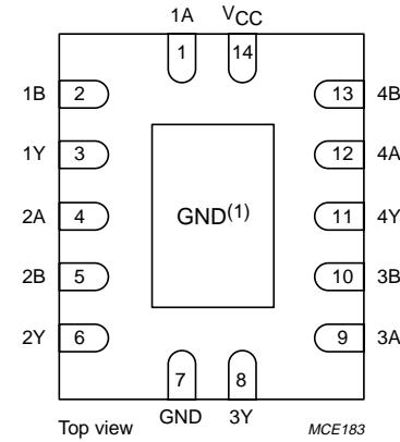
(1) The die substrate is attached to this pad using conductive die attach material. It can not be used as a supply pin or input.
