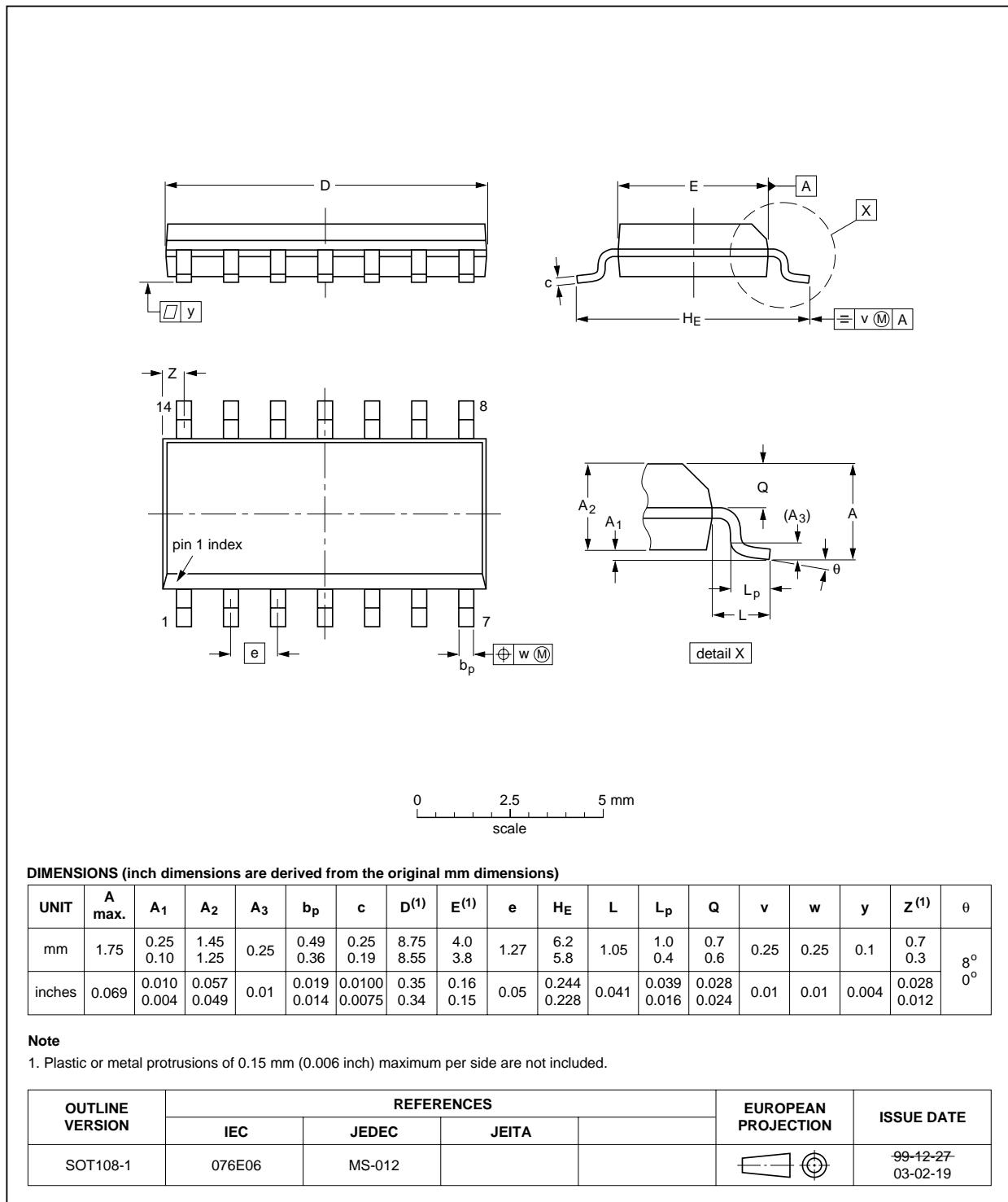
DIMENSIONS (inch dimensions are derived from the original mm dimensions)
