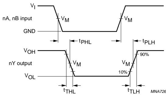
74HC08:  $V_M = 50\%$ ;  $V_I = \text{GND to } V_{CC}$ .74HCT08:  $V_M = 1.3$  V;  $V_I = \text{GND to } 3$  V.
