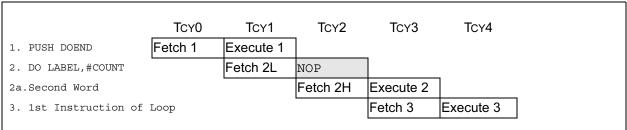
Instructions that are subjected to a stall due to a data dependency between the X RAGU and X WAGU. An additional cycle is inserted to resolve the resource conflict, as shown in Figure 2-8. Instruction stalls caused by data dependencies are further discussed in Section 4.0.
