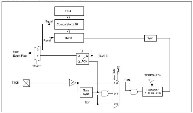
FIGURE 11-3: 16-BIT TIMER5 BLOCK DIAGRAM
