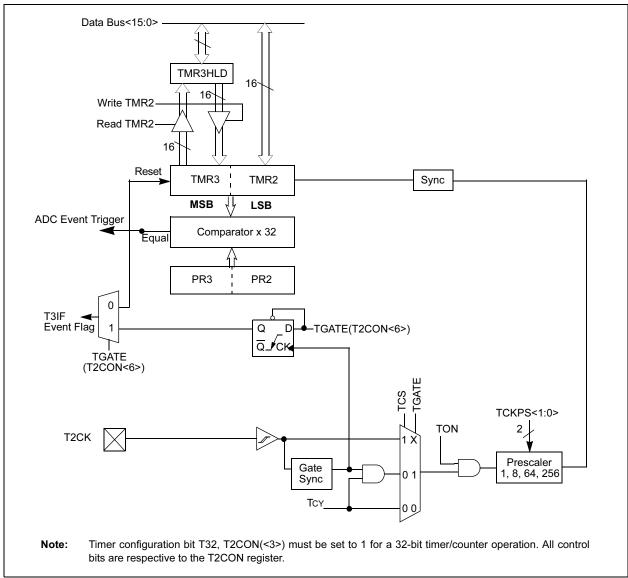
FIGURE 10-2: 16-BIT TIMER2 BLOCK DIAGRAM
