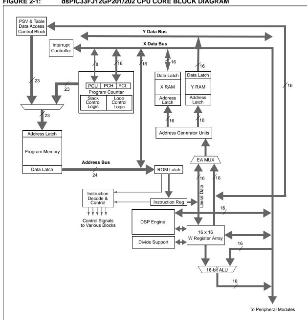
FIGURE 2-1: dsPIC33FJ12GP201/202 CPU CORE BLOCK DIAGRAM
