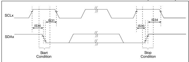
FIGURE 21-16: I2Cx BUS DATA TIMING CHARACTERISTICS (SLAVE MODE)
