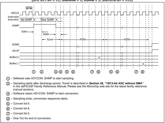
FIGURE 21-19: ADC CONVERSION (10-BIT MODE) TIMING CHARACTERISTICS (CHPS<1:0> = 01, SIMSAM = 0, ASAM = 1, SSRC<2:0> = 111, SAMC<4:0> = 00001)
