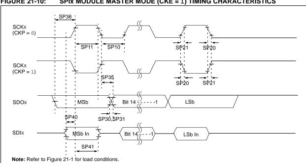
FIGURE 21-10: SPIX MODULE MASTER MODE (CKE = 1) TIMING CHARACTERISTICS
