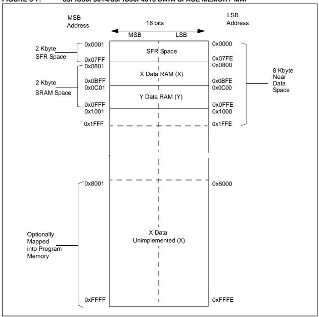
FIGURE 3-8: DATA SPACE FOR MCU AND DSP (MAC CLASS) INSTRUCTIONS EXAMPLE
