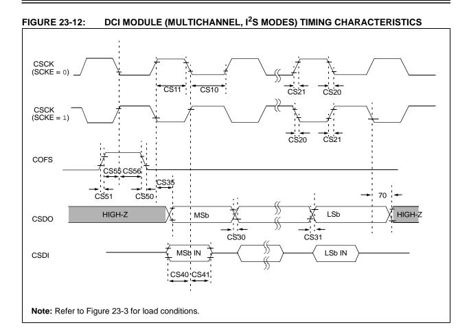
TABLE 23-28: DCI MODULE (MULTICHANNEL, I<sup>2</sup>S MODES) TIMING REQUIREMENTS
