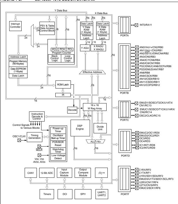
FIGURE 1-2: dsPIC30F4013 BLOCK DIAGRAM
