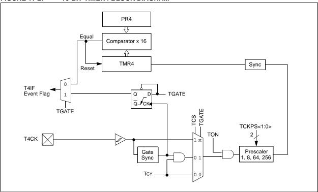
FIGURE 11-3: 16-BIT TIMER5 BLOCK DIAGRAM
