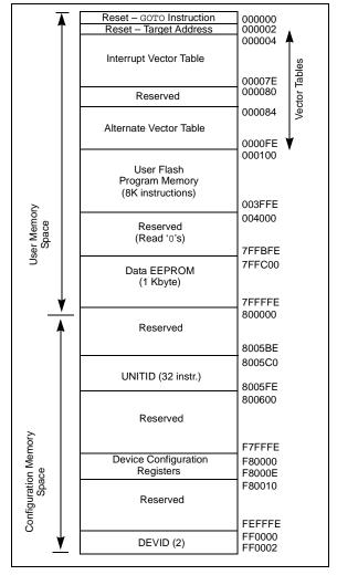
User program space access is restricted to the lower 4M instruction word address range (0x000000 to 0x7FFFFE) for all accesses other than TBLRD/TBLWT, which use TBLPAG<7> to determine user or configuration space access. In Table 3-1, bit 23 allows access to the Device ID, the User ID and the Configuration bits; otherwise, bit 23 is always clear.
