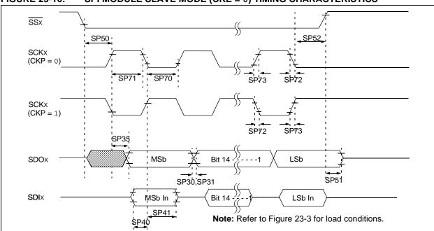
FIGURE 23-16: SPI MODULE SLAVE MODE (CKE = 0) TIMING CHARACTERISTICS
