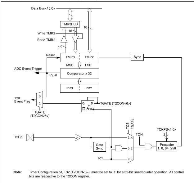
FIGURE 10-2: 16-BIT TIMER2 BLOCK DIAGRAM
