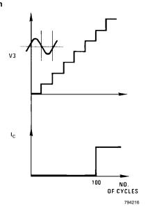
V3 steps up in voltage by the amount  $\frac{V_{CC} \times C1}{C2}$  for each complete input cycle (2 zero crossings) Example:
