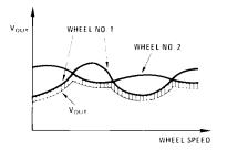
$m V_{OUT}$  is proportional to the lower of the two input wheel speeds.
