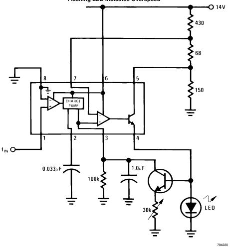
Flashing begins when  $f_{\rm IN} \ge 100$  Hz. Flash rate increases with input frequency increase beyond trip point.
