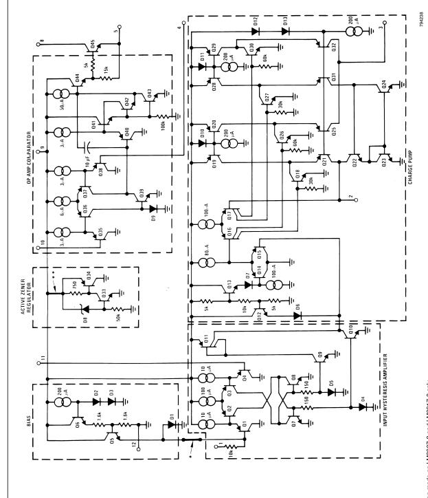
\*This connection made on LM2907-8 and LM2917-8 only. \*\*This connection made on LM2917 and LM2917-8 only.
