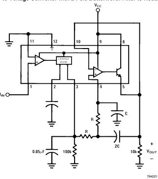
$$\begin{split} f_{\text{POLE}} &= \frac{0.707}{2\pi\text{RC}} \\ \tau_{\text{RESPONSE}} &= \frac{2.57}{2\pi\text{f}_{\text{POLE}}} \end{split}$$
