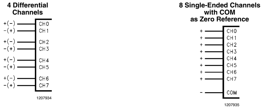
FIGURE 9. Input Multiplexer Options
