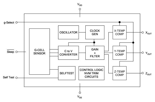
Figure 2. Simplified Accelerometer Functional Block Diagram
