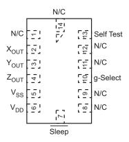
**Figure 4. Pinout Description**
