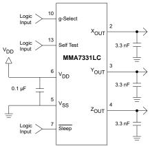
Figure 5. Accelerometer with Recommended Connection Diagram
