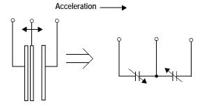
Figure 3. Simplified Transducer Physical Model SPECIAL FEATURES
