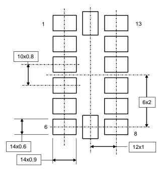
Figure 8. LGA 14-Lead, 5 x 3 mm Die Sensor
