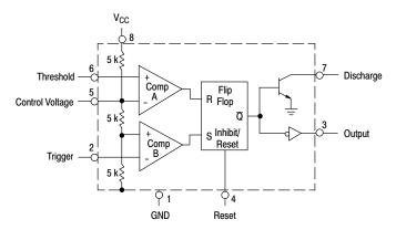
Figure 2. Representative Block Diagram
