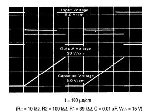
Figure 22. Linear Voltage Ramp Waveforms
