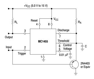
Figure 21. Missing Pulse Detector
