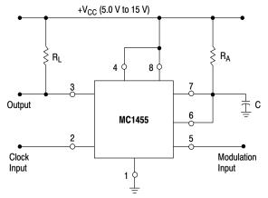
Figure 24. Pulse Width Modulator
