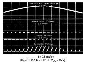
Figure 25. Pulse Width Modulation Waveforms
