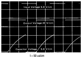
(RA = 10 k $\Omega$ , C = 0.01  $\mu$ F, RL = 1.0 k $\Omega$ , VCC = 15 V)
