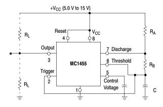
Figure 17. Astable Circuit
