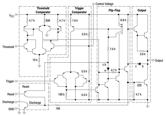
Figure 13. Representative Circuit Schematic
