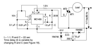
Figure 1. 22 Second Solid State Time Delay Relay Circuit
