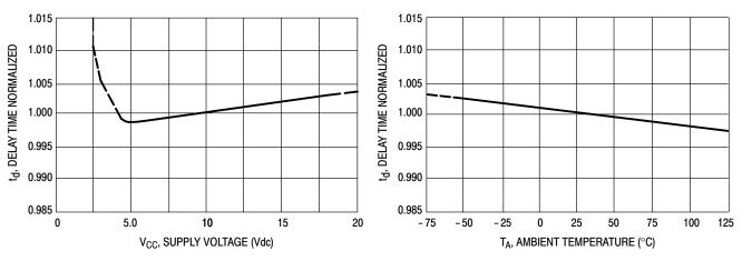
Figure 10. Delay Time versus Supply Voltage
