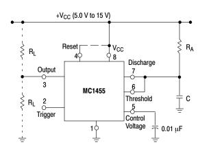
Figure 14. Monostable Circuit
