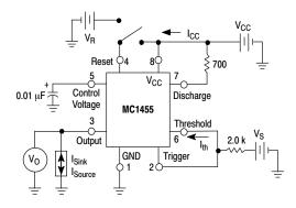
Test circuit for measuring DC parameters (to set output and measure parameters):
