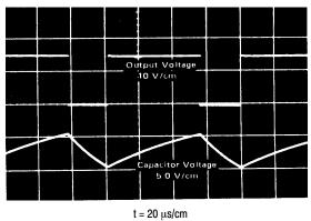
$(R_A = 5.1 \text{ k}\Omega, C = 0.01 \mu\text{F}, R_L = 1.0 \text{ k}\Omega; R_B = 3.9 \text{ k}\Omega, V_{CC} = 15 \text{ V})$
