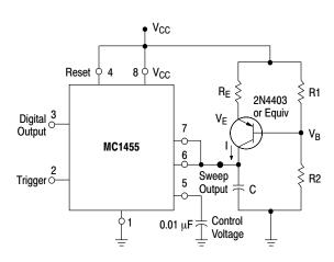
Figure 20. Linear Voltage Sweep Circuit
