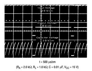
Figure 23. Missing Pulse Detector Waveforms
