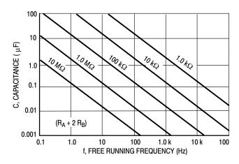
Figure 19. Free Running Frequency
