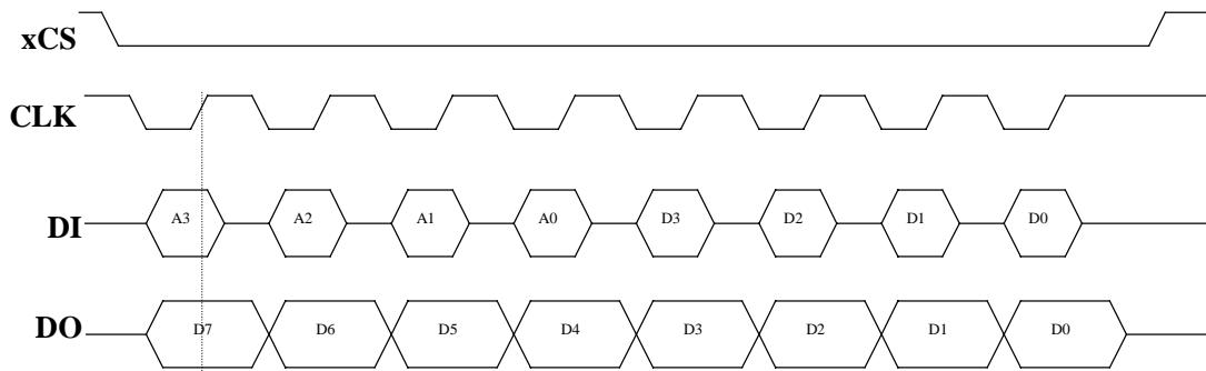
Note: The pins xCS,CLK,DI have internal pull-up resistors.
