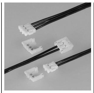
This ACH connector is compact and low profile type, height: 1.4mm (.055") and width 4.3mm (.169"), 1.2mm (.047") pitch wire-to-board connector.
