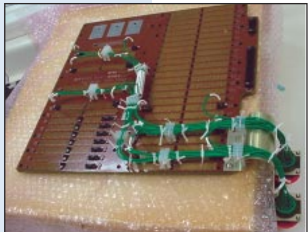
Harness composed of 25 fiber optic cable assemblies installed on a backplane for use in a missile fire control system.
