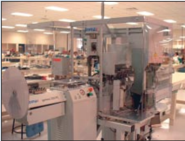
Komax automatic high-speed wire cutter/stripper/terminator, which makes complete single conductor wire assemblies.
