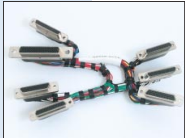
Military micro D-sub connectors, 100-pin and 50-pin, used in missile applications.
