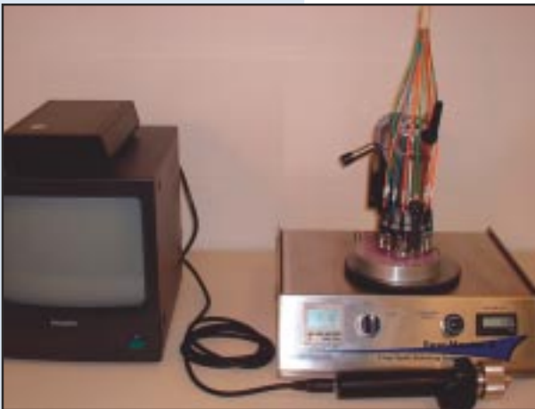
16 Station fiber optic auto-polisher and monitor ensures the quality of a polish on the fiber face.
