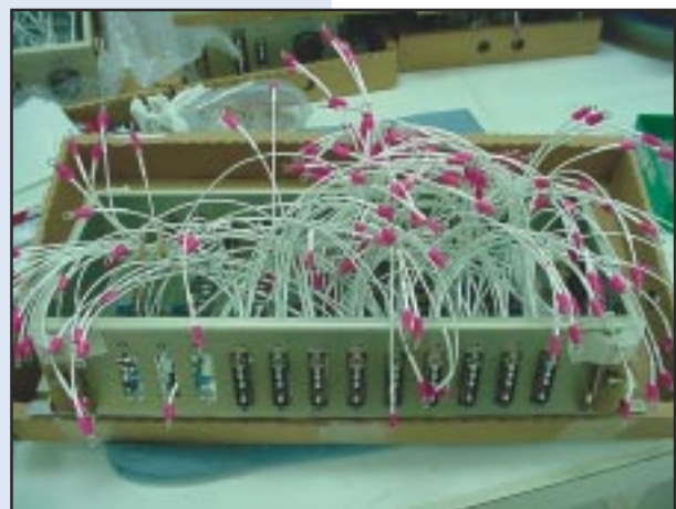
This 270-volt distribution box is an example of the complex box-builds capable by WPI.
