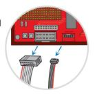
2. On the EM35x NCP Breakout Board: attach ISP Cable to InSight Port and DEI Cable to DEI Port.
