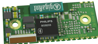
Picture 2: CB-OEMSPA311i-07 OEM Serial Port Adapter short range with internal antenna and a flexfilm connector
