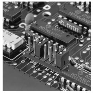
This is a two-circuit jumper connector suited for changing or switching circuits on printed circuit boards without using DIP switches. It is compact and light, thus can be mounted on printed circuit boards without interfering with the placement of other components. The connector is easy to use, low in cost, and has a wide range of applications in industrial and consumer products.
