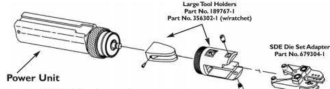
Part No. **189721-1** (hand actuated) Part No. **189722-1** (foot actuated)
