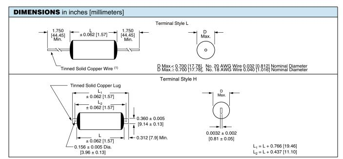
Note (1) Leads to be within ± 0.062" [1.57 mm] of center line at egress but not less than 0.031" [0.79 mm] from edge (Terminal Style L only).
