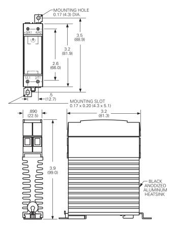
Recommended Torque Range for Terminal Screws: 5 - 6 in lb (0.6 - 0.7 Nm).
