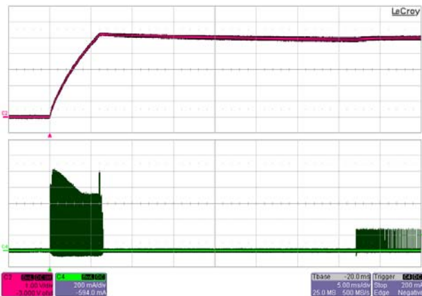
Figure 28 – No-load at 127 VDC Input Voltage Upper: V_{STBY} , 1 V / div. Lower: Standby I_{DRAIN} , 200 mA, 5 ms / div.
