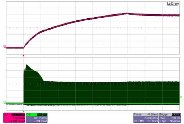
Figure 27 – Full Load: 380 VDC Input Voltage. Upper: V_{STBY} , 1V / div. Lower: Standby I_{DRAIN} , 200 mA, 2 ms / div.
