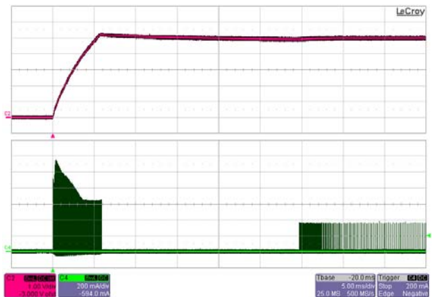
Figure 29 – No-load at 380 VDC Input Voltage Upper: V_{STBY} , 1 V / div. Lower: Standby I_{DRAIN} , 200 mA, 5 ms / div.
