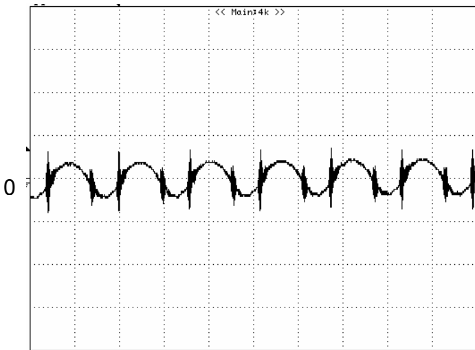
Figure 12: Input reflected ripple current, i_s , through a 12\mu\text{H} source inductor at nominal input voltage and rated load current ( 20\text{ mA/div} , 2\mu\text{s/div} )
