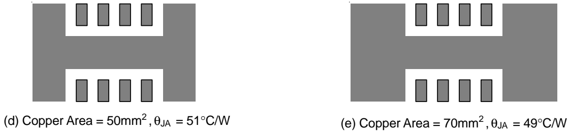
Figure 6. Thermal Resistance vs. Copper Area Layout Design
