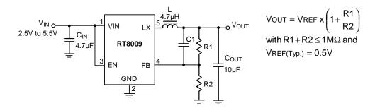
Figure 2. Adjustable Voltage Regulator
