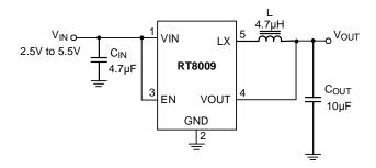
Figure 1. Fixed Voltage Regulator
