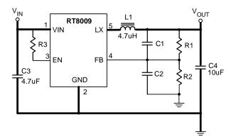
Figure 6. EVB Schematic
