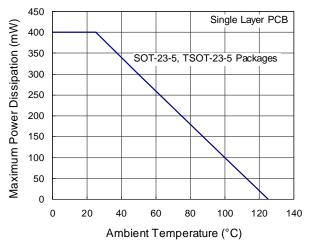
Figure 5. Derating Curves for RT8009 Package
