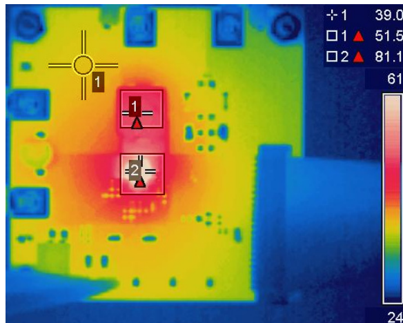
Figure 18: Thermal Image at V_{IN} = 12V , I_{OUT} = 10A (IR3865: 81^\circ C , Inductor: 52^\circ C , PCB: 39^\circ C )
