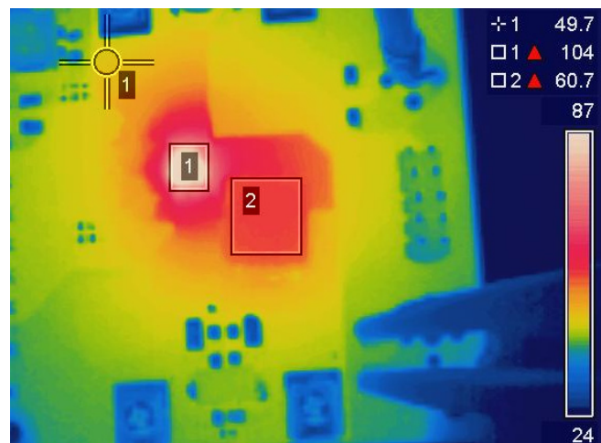
Figure 22: Thermal Image at VIN = 19V, IOUT = 12A (IR3476: 104°C, Inductor: 61°C, PCB: 50°C)
