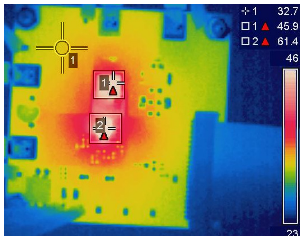
Figure 19: Thermal Image at V_{IN} = 16V , I_{OUT} = 6A (IR3863: 61^\circ C , Inductor: 46^\circ C , PCB: 33^\circ C )
