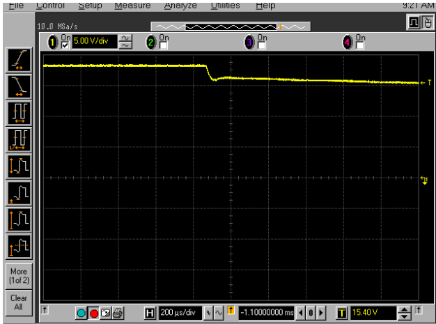
FIGURE 10. VLNb TRANSITIONS FROM 18.3V TO 13.3V
