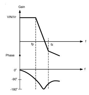
Figure 7. The Bode plot of Buck power stage
