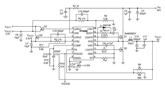
Figure 2. Typical Application for 24V Input
