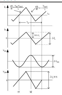
Figure 2. The related waveforms of output capacitor.
