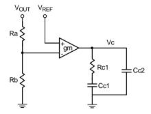
Figure 9. The typical type 2 trans-conductance error amplifier.
