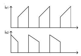
Figure 1.The waveforms of synchronous step-down converter
