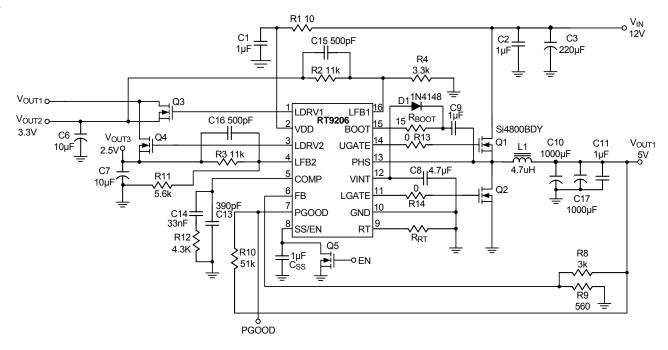
Figure 1. Typical Application for 12V Input
