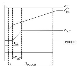
Figure 4. The soft-stat timing diagram of RT9206
