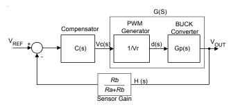
Figure 6. The control block diagram of synchronous Buck converter
