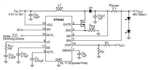
Figure 2. PWM to Analog Dimming in Boost Configuration
