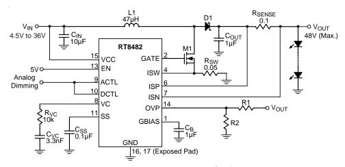
Figure 1. Analog Dimming in Boost Configuration
