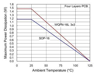
Figure 5. Derating Curves for RT8482 Packages
