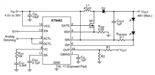
Figure 3. Analog Dimming in Buck-Boost Configuration
