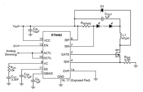
Figure 4. Analog Dimming in Buck Configuration
