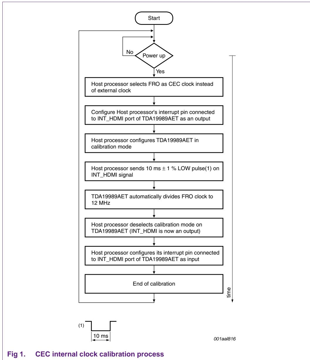
Fig 1. CEC internal clock calibration process
