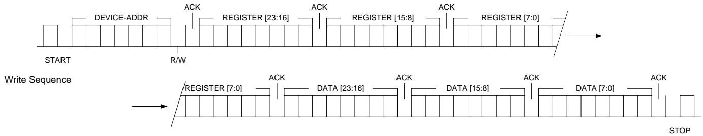
FIGURE 14. I 2 C WRITE SEQUENCE OPERATION
