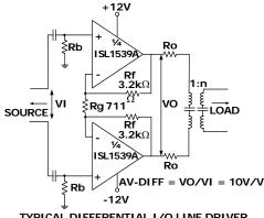
TYPICAL DIFFERENTIAL I/O LINE DRIVER (1 OF 2 PORTS)
