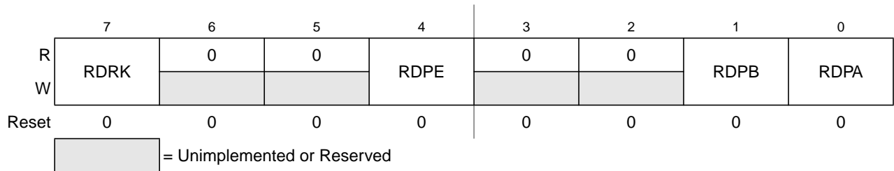
Figure 21-15. Reduced Drive Register (RDRIV)
