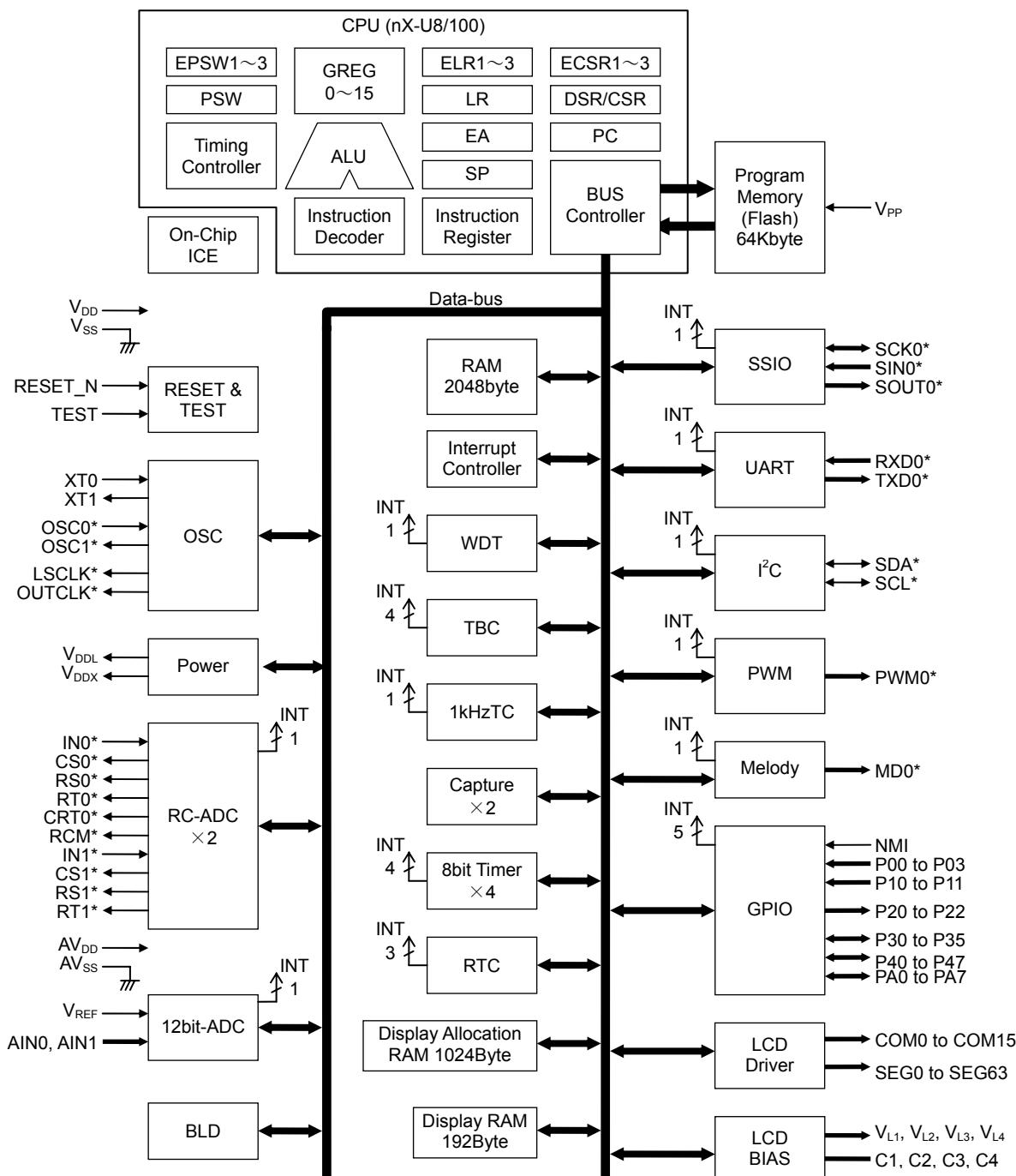
**Figure 1 ML610Q431 Block Diagram**
