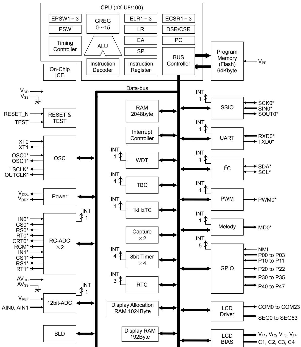
Figure 2 ML610Q432 Block Diagram
