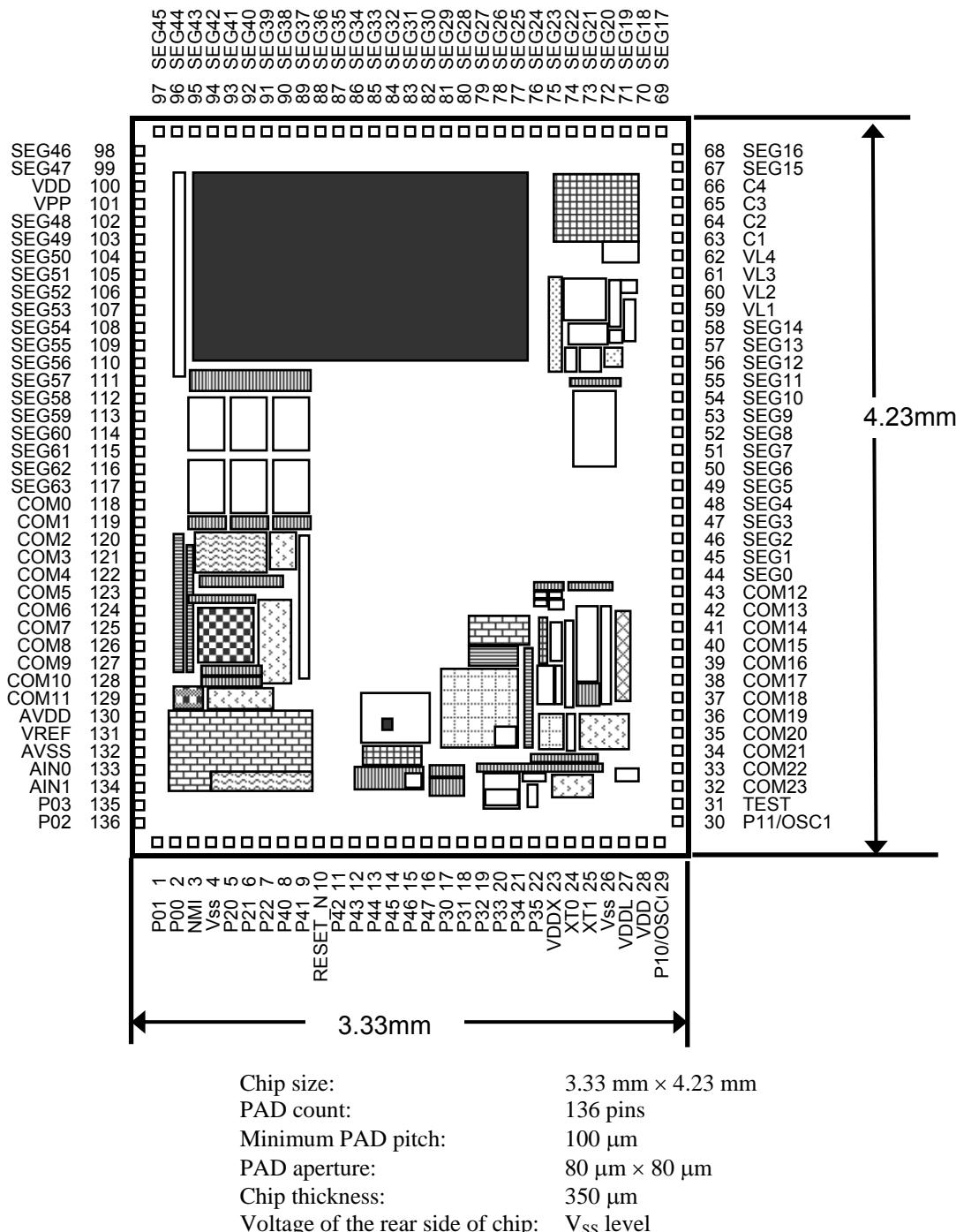
Figure 6 ML610Q432 Chip Layout &amp; Dimension
