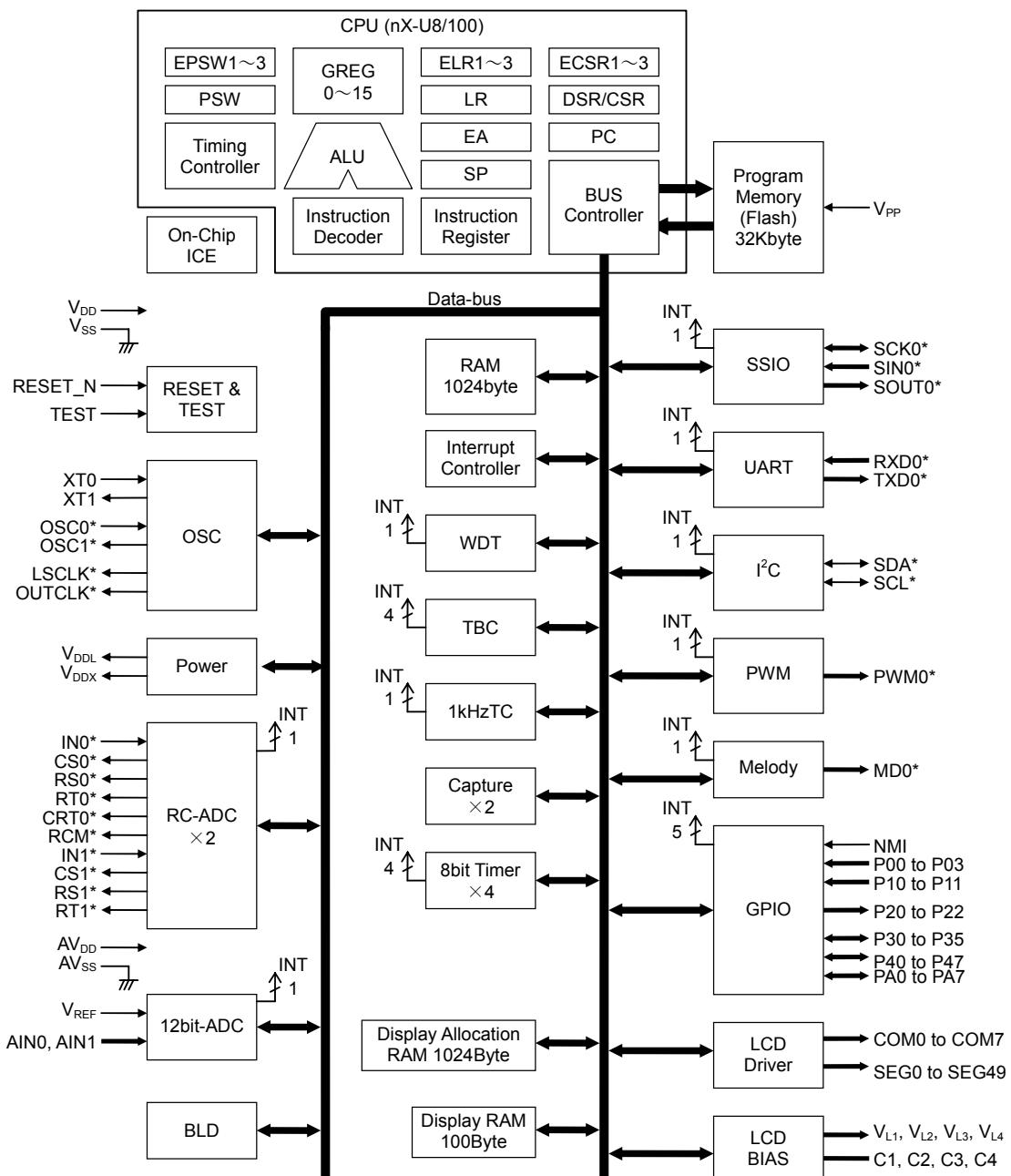
**Figure 1 ML610Q421 Block Diagram**
