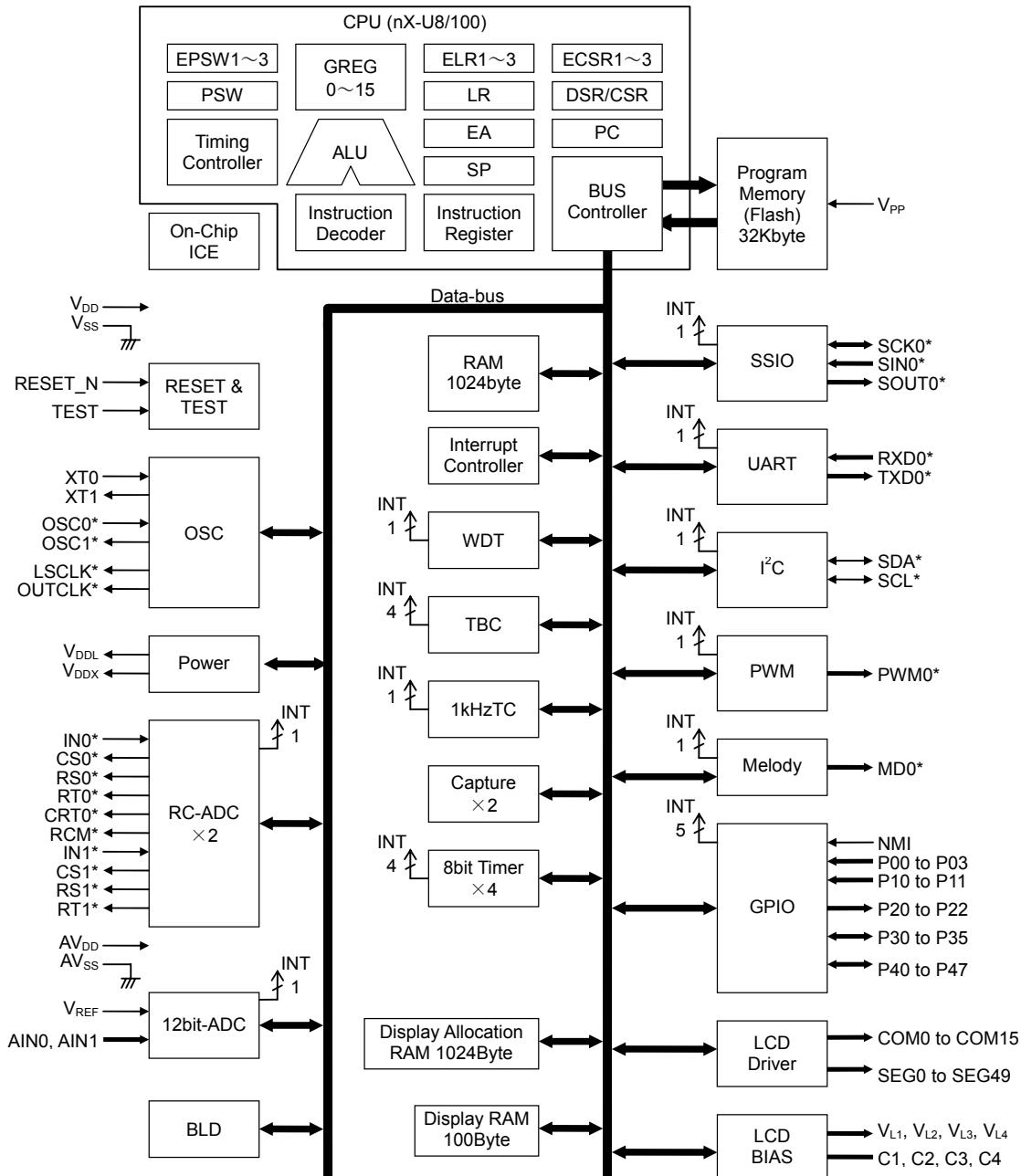
**Figure 2 ML610Q422 Block Diagram**
