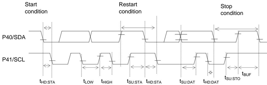
**AC CHARACTERISTICS (RC Oscillation A/D Converter)**
