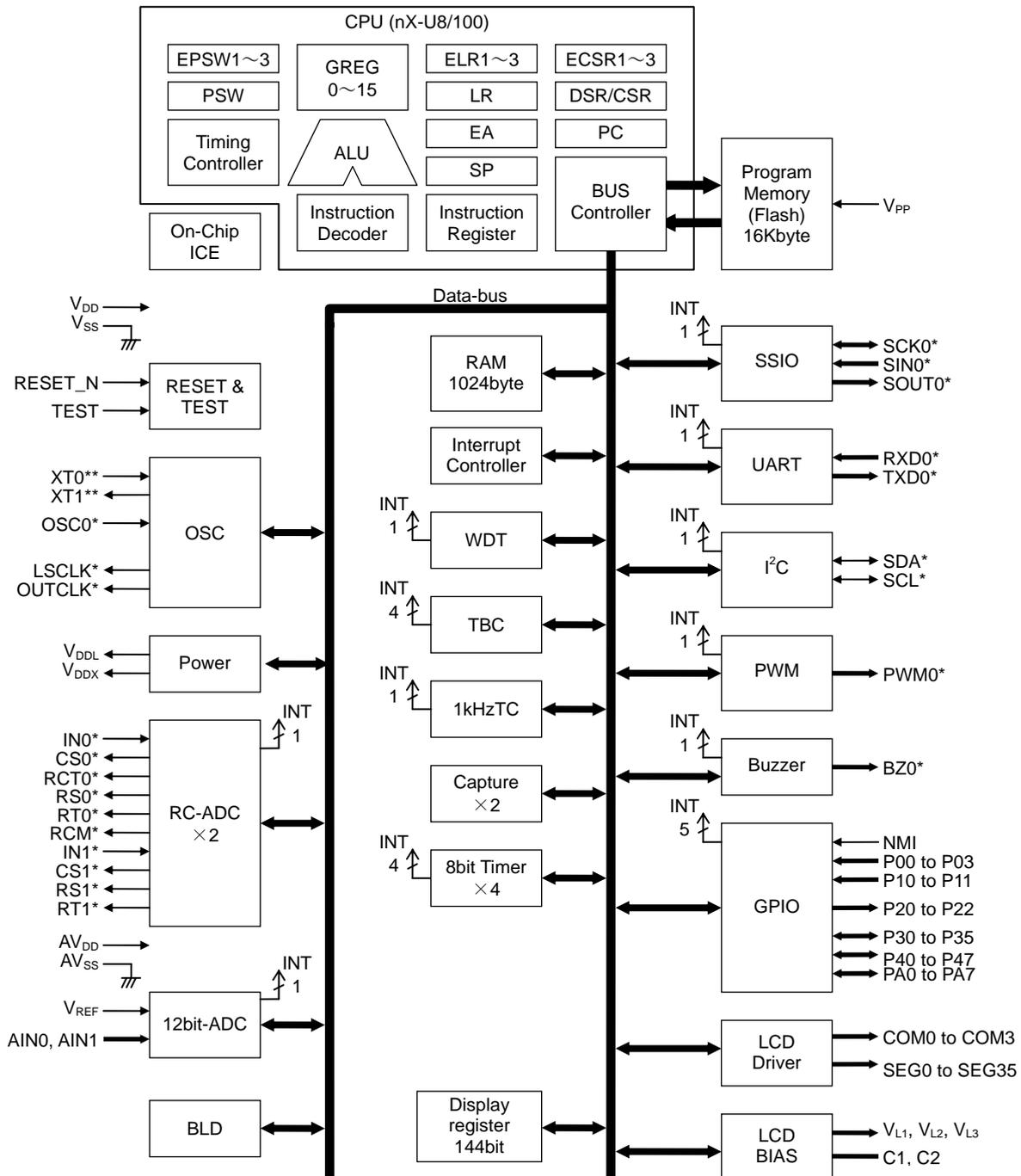
Figure 1 ML610Q411/ML610Q415 Block Diagram
