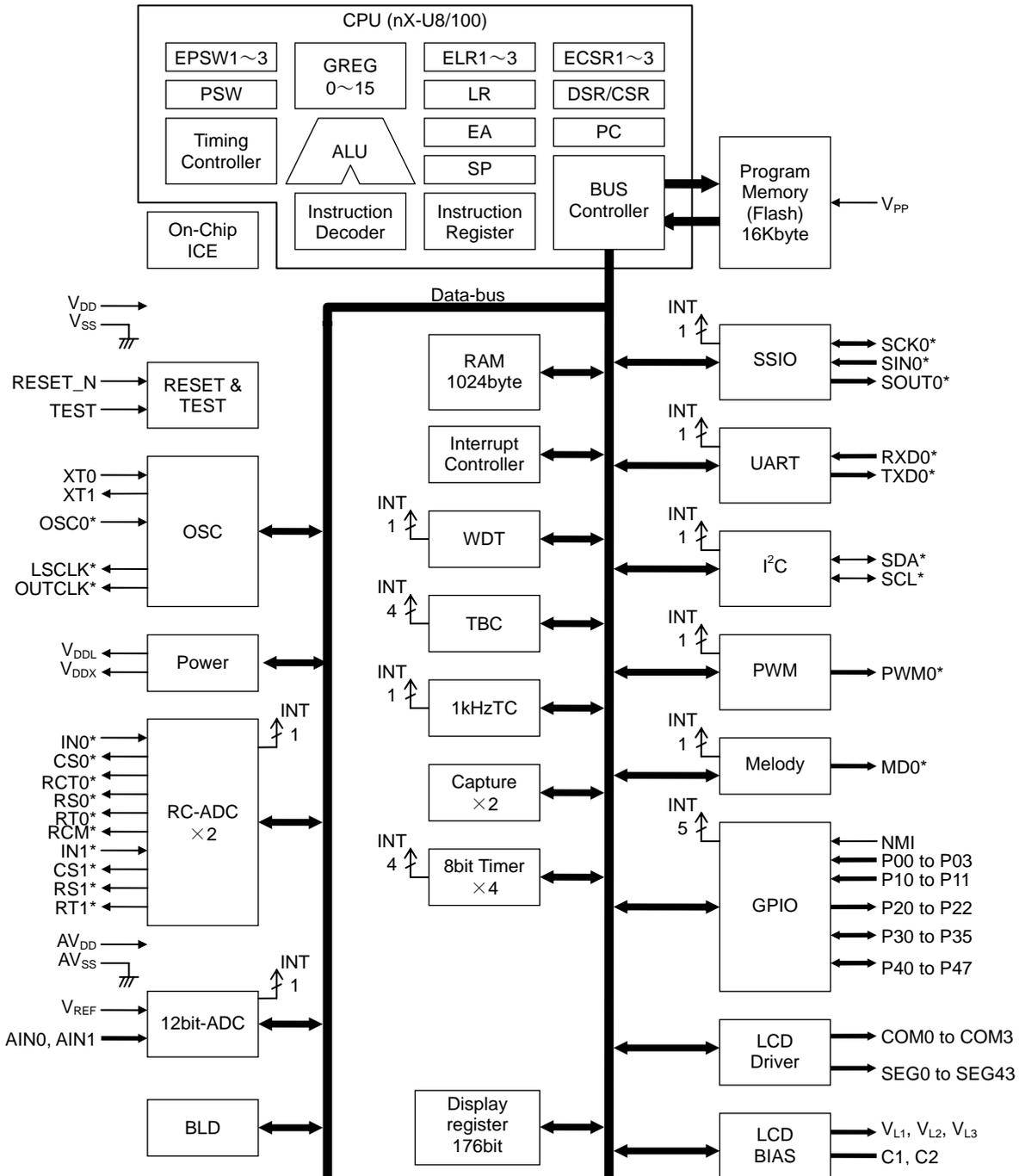
**Figure 2 ML610Q412 Block Diagram**
