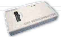
Compact, lightweight debugging emulator μEASE (50mm×90mm×9mm 50g)
