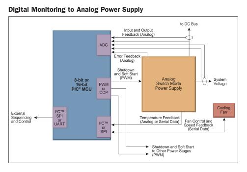
soft-start profiles and current limits can be programmed to suit the application. The output voltage can be fine-tuned to provide coordination between multiple power supplies in a system. Depending on the system I/O requirements, 8-bit solutions in the PIC12, PIC16 or PIC18 device families can provide the ideal solution. In larger systems, the 16-bit PIC24 device family can provide more communication peripherals.
