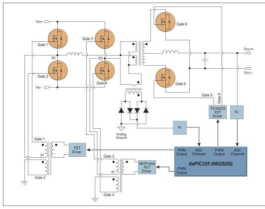
The dsPIC33FJXXGS DSC family in power efficient and highly integrated DC-DC converters dynamically controls different power stages. Highspeed ADC, PWM and comparators work together without using much CPU bandwidth. Faster digital control loops and compensators can be executed using a high-performance DSP engine. Advanced features such as dynamic load response, protections, sequencing, remote control and communications can also be implemented.
