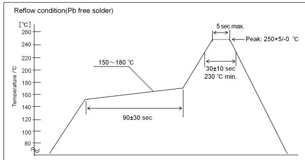
The products may be exposed to reflow soldering process of above profile up to two times.
