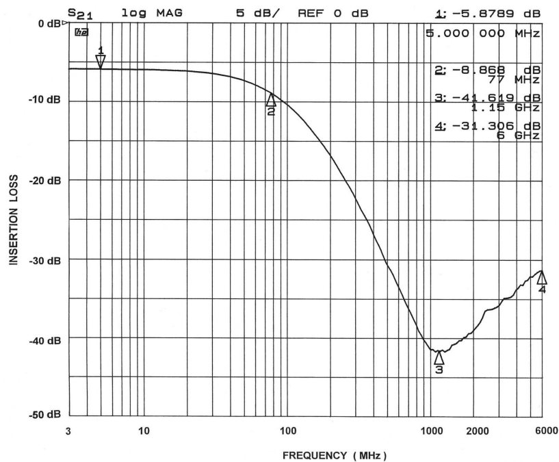
Figure 1. A1-C1 EMI Filter Performance
