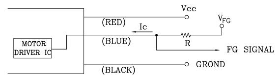
CAUTION: THE RD SINGAL LEAD WIRE MUST BE KEPT AWAY FROM "+" LEAD WIRE & "-" LEAD WIRE.
