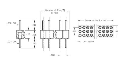
Description: Interconnect Header .100 Grid; Straight Pin Header .030 Pin Head with Solder Tail; Low Profile Triple Row Through Hole Plating Code: 10
