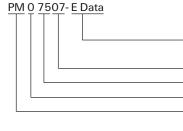
Copy Type (Blank, E Data, or Hard Data) Tag height (mm) Tag length (mm) Filler character Permark<sup>®</sup>
